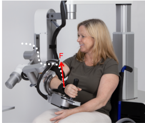
Figure 1.2: Representative figure of assisting. White dots shows the desired position over time. Red line represents the assistance by the exoskeleton
