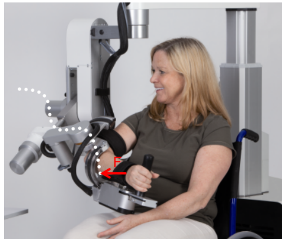
Figure 1.3: Representative figure of correcting. White dots shows the desired position over time. Red line represents the correcting force applied by the exoskeleton
