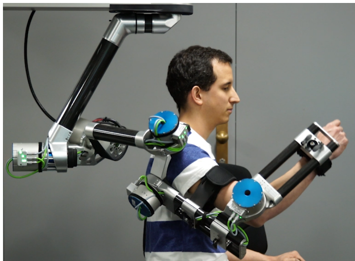
Figure 2.1: Exoskeleton arm of ANYexo with a user [1].
